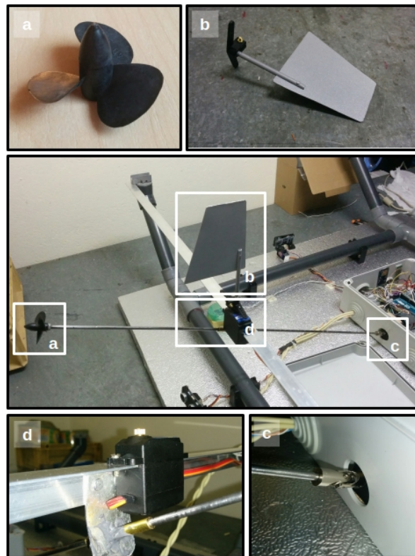
Figure 8. Main mechanical elements for propulsion and direction: (a) 3-blade propeller; (b) Rudder; (c) steel transmission shaft; (d) and waterproof servo for rudder control.
