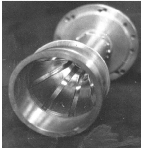
Fig. 15. Relativistic magnetron with diffraction output, an alternative approach to RF extraction.
