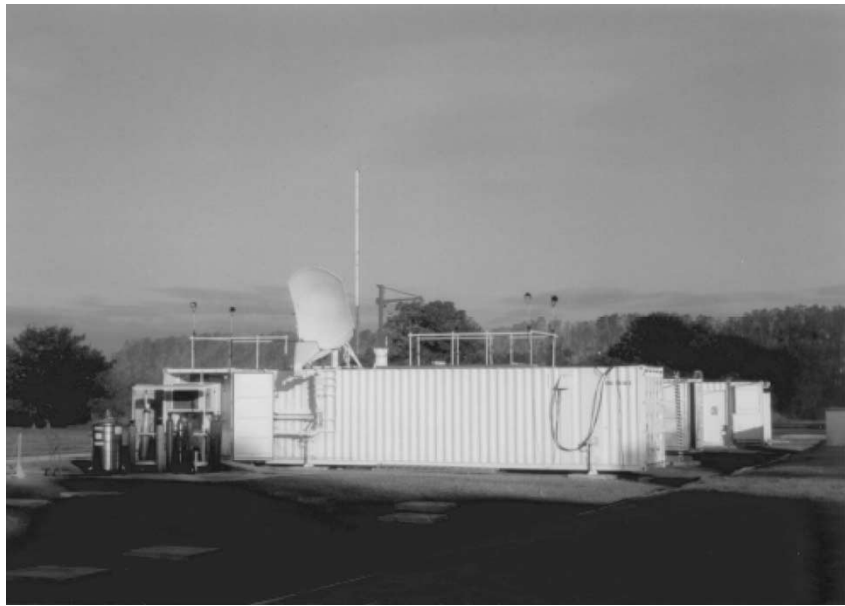
Fig. 14. HPM test facility ORION (manufactured by Titan/Pulse Sciences Division), which is based on a series of relativistic magnetrons.
